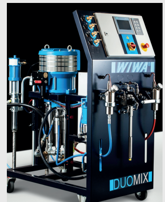
WIWA DUOMIX, pneumatic plural component spray equipment
